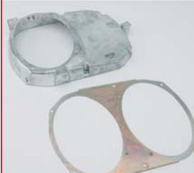
1970-74 Blower Speaker Housing. Defrost/Speakaer under Package Tray
